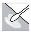
1. The test solution is applied to the surface of the sample representing the lot of passivated parts, applying additional solution if needed to keep the surface wet for a period of at least six minutes.
