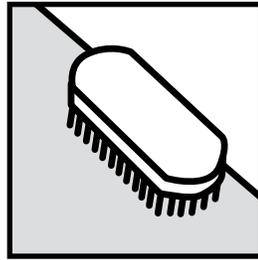
**3.** Remove loose scale with a stainless steel or plastic bristle brush. For exceptionally heavy scale, repeat the process.
