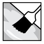
1. Apply a thick layer using an acid resistant brush or applicator. Paste may settle during shipment. Stir to thicken.
