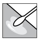
1. Apply a thick layer of Wonder Gel with an acid resistant brush or other appropriate applicator. Room temperature or warmer is recommended.
