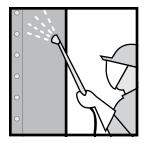
1. Dip, spray or brush the Derustit SS-3™. Using a plastic container, immerse the surface to be treated into a bath of Derustit SS-3™ liquid.
